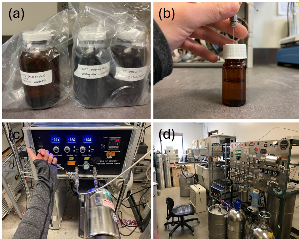
Figure B14. The procedure of headspace analysis to characterize drilling mud fluid outgassing. A series of headspace VOC analyses of both pure Neoflo drilling fluid and of a recycled drilling mud sample were conducted in the CSU lab.
