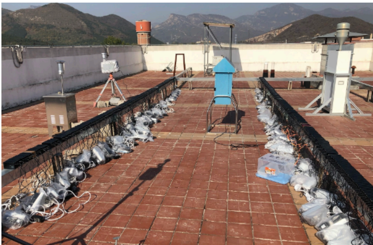
Figure 2. Calibration of real-time sensors against a reference monitor at the University of the Chinese Academy of Sciences.
