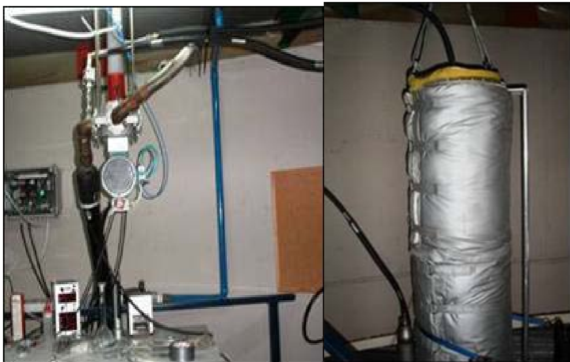
Figure 16. Setup of valve-denuder-chamber effluent tubing during injection, arrow indicates chamber entrance line (left panel), and denuder with heating mantel (right panel), secured below the chamber.
