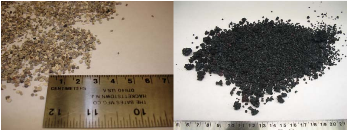
Figure 3. GROG before (left) and after (right) coating with cobalt oxide.
