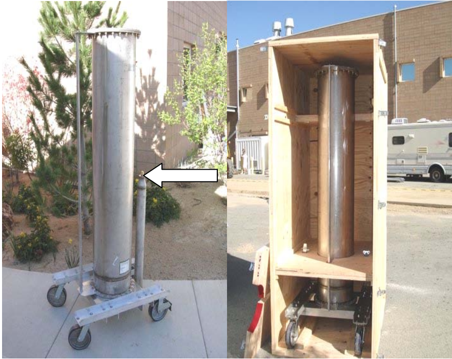
Figure 15. Denuder mounted on wheeled base (left panel) with effluent entrance elbow visible (arrow), and denuder inside specially constructed transportation crate (right panel).
