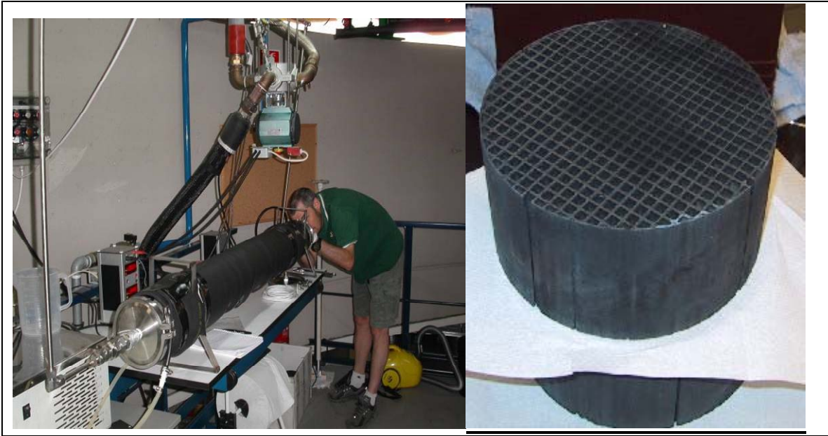
Figure 1. Cordierite honeycomb NO x denuder used in summer 2005. Left panel: NO x denuder installed in EUPHOR facility; right panel: honeycomb structure of one ceramic piece, coated with cobalt oxide.
