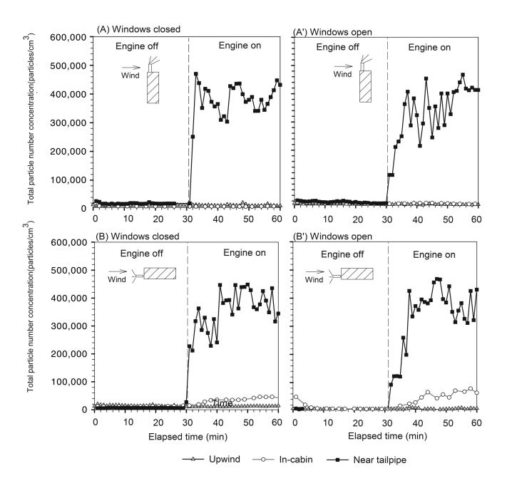
**Figure A.8.** Typical time series of PNCs in the upwind air, in-cabin air, and air close to the tailpipes under scenarios C and D with different window positions. Shaded boxes indicate the buses in which the measurements were shown. Rays indicate the buses of which the engines were turned on.
