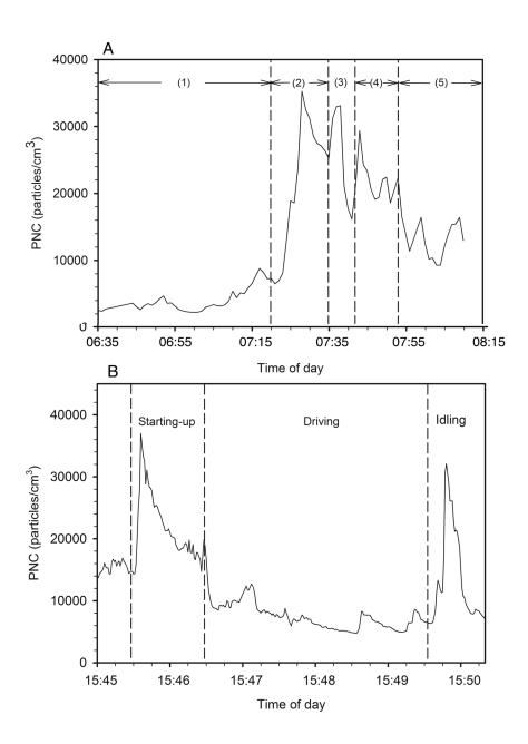
**Figure A.7.** Typical time series of PNCs in the upwind air, in-cabin air, and air close to the tailpipes under scenarios A and B with different window positions. Shaded boxes indicate the buses in which the measurements were shown. Rays indicate the buses of which the engines were turned on.
