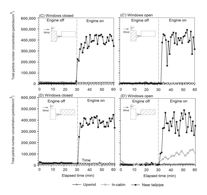
**Figure A.9.** Typical time series of PNCs in the upwind air, in-cabin air, and air close to the tailpipes under scenario E with different window positions. Shaded boxes indicate the buses in which the measurements were shown. Rays indicate the buses of which the engines were turned on.
