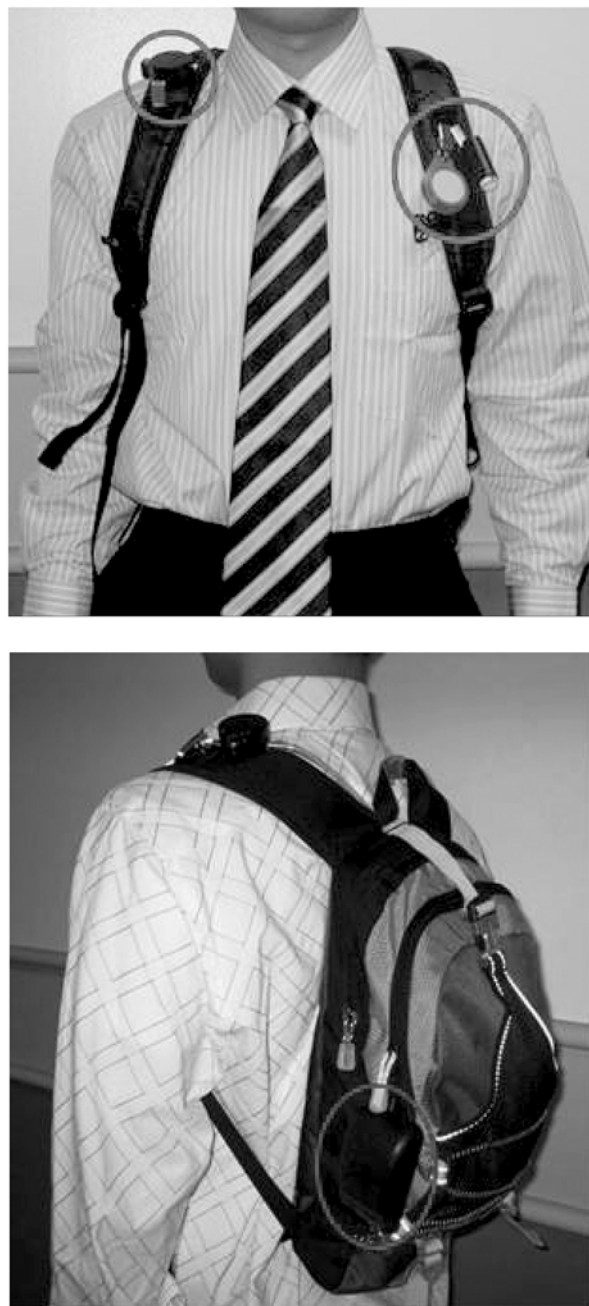
Figure 2. Sampling backpack on a subject. Front view (top) shows the personal exposure monitors on the shoulder straps and the pump in the backpack. Back view (bottom) shows the GeoLogger receiver hanging outside the backpack.
