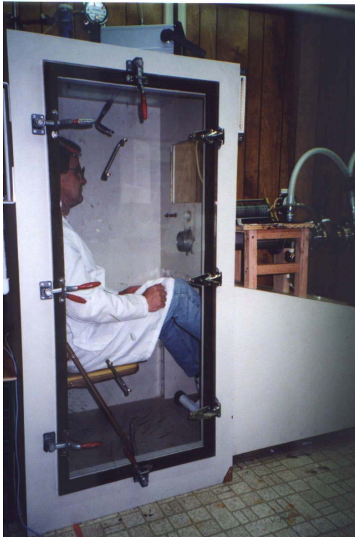
Figure D-3. Side view of exposure chamber with staff member inside in subject's usual position. (Actual subjects wore clean-room clothing when inside.) Inlet pipe (larger opening) and main (MOUDI) sampling port (smaller opening) are visible in front wall below window. Sampling instrument platform and hoses of HEPA-filter-containing bypass circuit are visible outside upper front of chamber.
