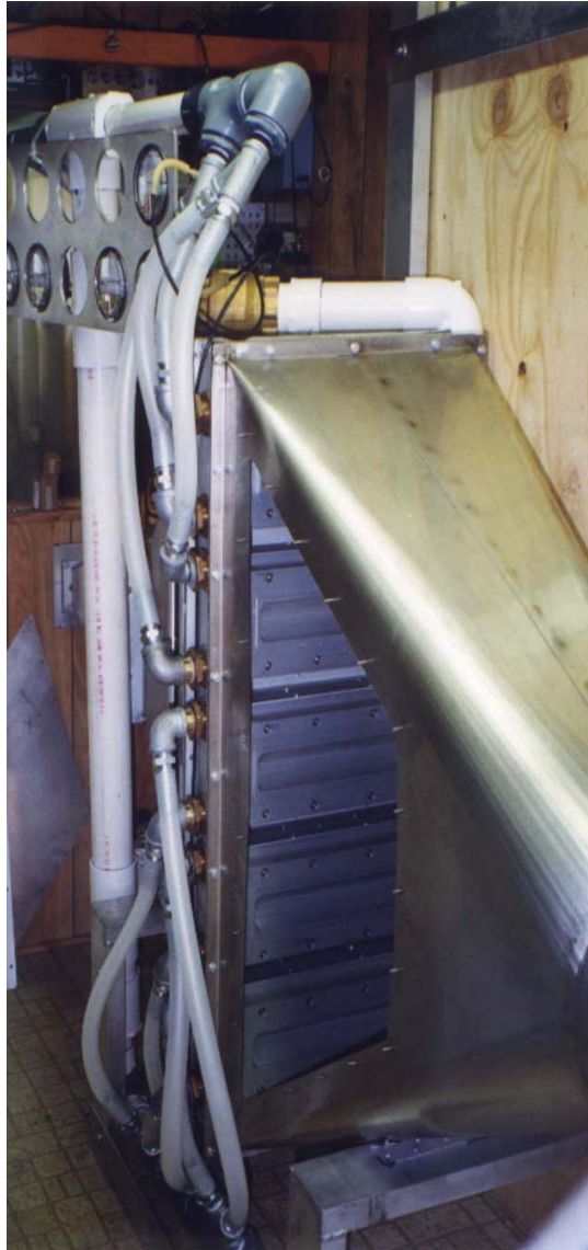
Figure D-2. Concentrator stage 1, viewed from upstream side with access hatch removed to show 5 impactor slits in parallel. Major flow exhaust hoses are visible to left of impactor slits.
