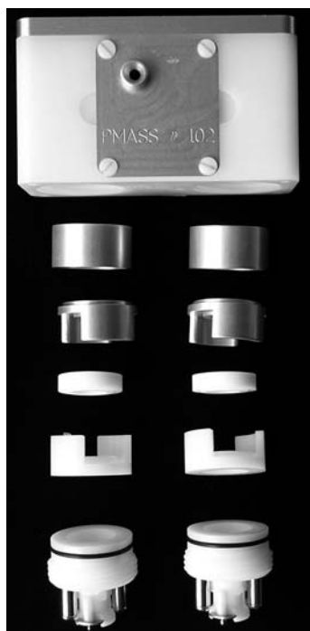
Figure 3. Exploded view of the PMASS. From top to bottom: sampler body, aluminum denuder rings, filter cassette components—aluminum caps, Teflon spacer disks, and Delrin bases—and end caps.
