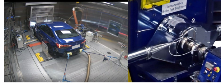
Zero-Emission Vehicle Brake-Wear Emissions Reduction Laboratory testing comparing emissions from gasoline and electric vehicles
