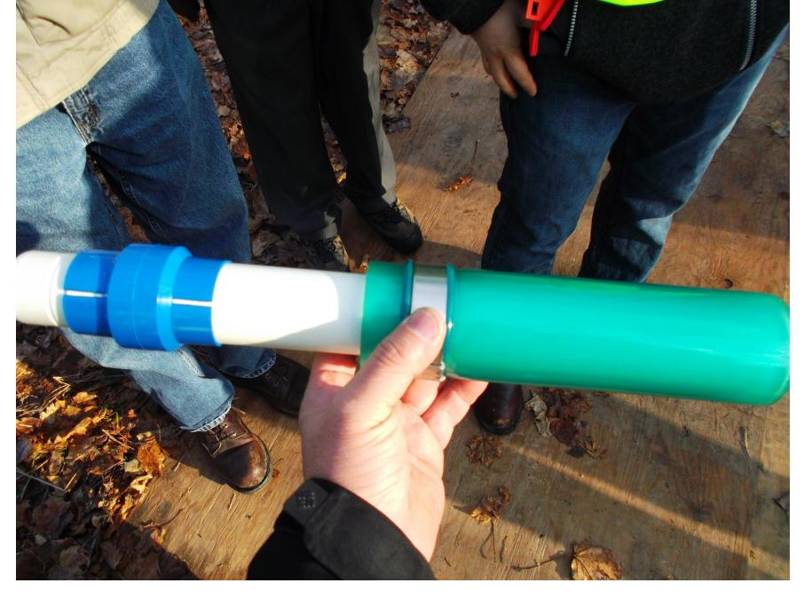
Multilevel sampler port with packer system for isolating aquifer flow zones.
