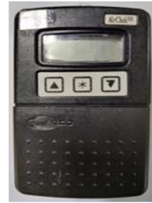
Air-check XR 5000 Active PM Sampler
