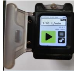
Air-check Touch Active PM Sampler
